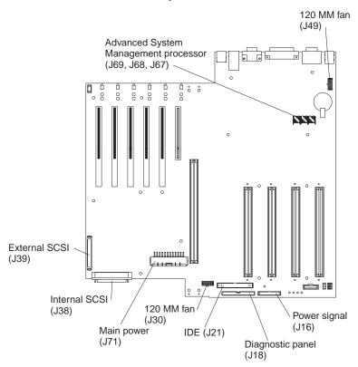
*I/O external port connectors:* The following illustration shows the location of the input/output external port connectors on the system board.
